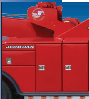
Lightweight, Corrosion-Proof, Bonded Composite & Aluminum Body
