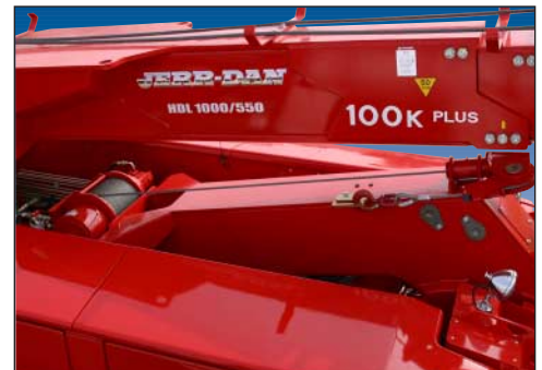
Optional Underlift Mounted Planetary Drag Winch Complete With 360° Swivel Cable Guide
