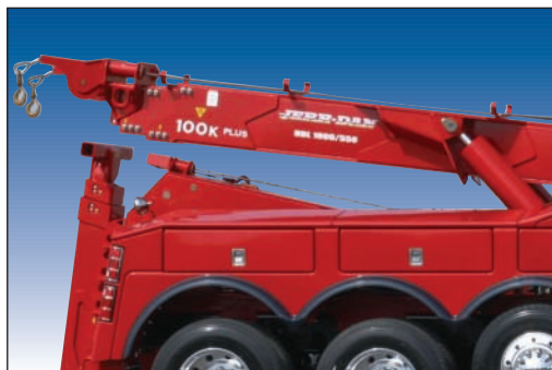
Fabricated Hi-Tensile Steel Recovery Boom Available in Both 2 and 3 Stage Configurations
