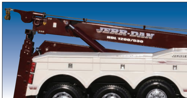
Fabricated Hi-Tensile Steel Recovery Boom
