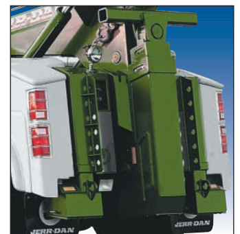
Independently Operated Three Stage Underlift
