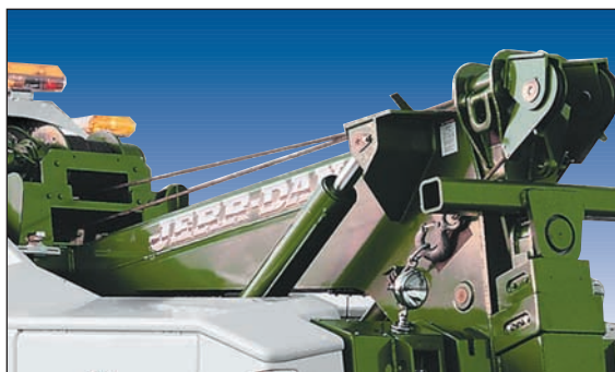
Fabricated Hi-tensile Steel Recovery Boom
