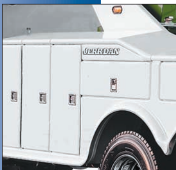
Lightweight, Corrosion-Proof, Bonded composite & Aluminum Body
